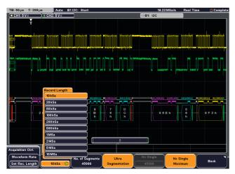
Capture and analyze pulsed and burst signals over a long period. 460 Msample deep segmented memory is unique in this class.
