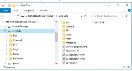
With the USB MTP implementation, you can easily access live channel data and screenshots and integrate the oscilloscope into your computing environment
