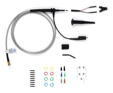
The R&S®RT-ZPR20 power rail probe is compatible with the R&S®RTO and the R&S®RTE digital oscilloscopes. The R&S®RTE (frequency range from 200 MHz to 2 GHz) is an economical deep memory solution with advanced functionality. The R&S®RTO (frequency range from 600 MHz to 6 GHz) offers a solution with more headroom. Both oscilloscopes achieve fast update rates of up to 1 million waveforms/s, providing greater power rail characterization confidence faster.
