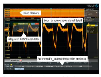
Time domain views of power rails to measure ripple, noise and transient.
