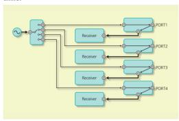
Block diagram of the per-port architecture
