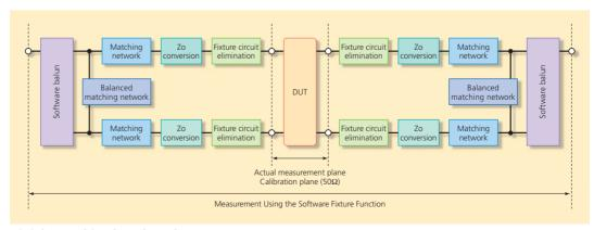
Block diagram of the software fixture function
