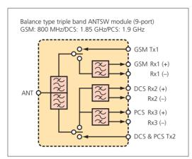
Example of a triple-band antenna switch module
