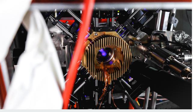
The image shows the strontium optical lattice clock under development at the University of Birmingham. Lasers and magnetic fields cool the atoms to a temperature a fraction above absolute zero and trap them inside a vacuum chamber. This allows the researchers to probe very precise transitions between energy levels in the strontium atoms, which provides the frequency reference for the optical atomic clock.
