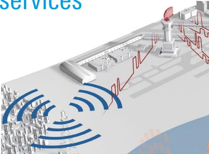
Coexistence testing of radars in the spectral vicinity of base stations or mobile phones requires a mix of communications signals and radar signals. S-band navigation radars operating in the spectral vicinity of LTE base stations or a mobile phone are a typical example. The performance of the radar receiver must be tested against this interference scenario.
