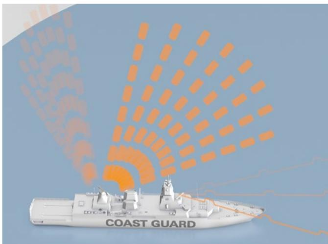
Emitters are transmitting stations that are characterized through items such as basic pulses with or without modulation on pulse (MOP), a sequence of the defined pulses, antenna diagram, antenna scan type and equivalent isotropically radiated power (EIRP). Emitters often have a variety of modes using a combination of the items mentioned above. The R&S®Pulse Sequencer software provides these simulation items for simulating complex 3D scenarios for receiver tests.
