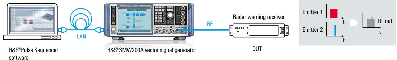
This setup is good for testing a single-channel radar receiver (DUT) in the frequency range up to 40 GHz with 2 GHz signal bandwidth and overlapping pulses (pulse-on-pulse signals). For this application, the R&S®SMW200A vector signal generator has two integrated baseband generators to generate the pulse-on-pulse signal through internal addition of the baseband signals.
