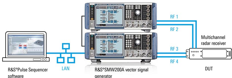
This setup is good for simulating angle of arrival (AoA) of emitters with two coupled dual-path R&S®SMW200A vector signal generators.
