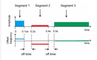
Achieve ultralong playtimes with realtime calculations that can adjust the amplitude, phase and frequency of the pulses. Realtime sequences can be created in the R&S<sup>®</sup>Pulse Sequencer software with the R&S<sup>®</sup>SMW200A UI or by importing .xml files.
