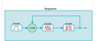
Powerful sequencer tools make it easy to create pulse sequencing that ranges from simple to complex. Combine different pulses, with different PRIs, frequencies and power levels for a truer real-life test signal.
