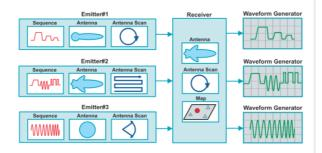
Build a complete scenario to simulate what an operational receiver would see. Multiple emitters with independent sequences and antenna profiles can easily be created and put together for a lifelike scenario. The software also allows location, frequency and power levels to be independently set.
