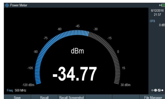
Power measurement using the internal power meter
