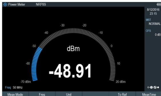
Power measurement with the R&S®NRP8S power sensor
