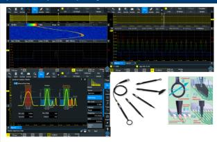
Difficult-to-find faults often result from the interaction between time and frequency signals. The R&S®RTx-K37 spectrum analysis and spectrogram option quickly finds such errors. Parameters such as center frequency and resolution bandwidth can be easily adapted to the specific measurement task. The oscilloscope automatically selects the relevant time domain settings.
