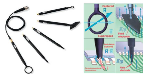
Powerful E and H near-field probes for the frequency range from 9 kHz to 3 GHz with an optional preamplifier expand the application range of the R&S®RTx-K37 spectrum analysis and spectrogram option to include EMI debugging.
