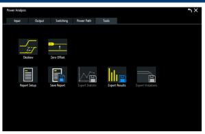
Add each result to the test report by simply pressing a button. The test report documents the setup and configuration. Define the level of detail in the report and customize the layout, for example by adding a company logo. The output format is PDF.
