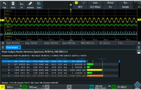
Different standards for limiting the harmonic current must be met when developing switched-mode power supplies. The R&S®RTx-K31 power analysis option helps you test all common standards: EN 61000-3-2 classes A, B, C, D, MIL-STD-1399 and RTCA D0-160.
