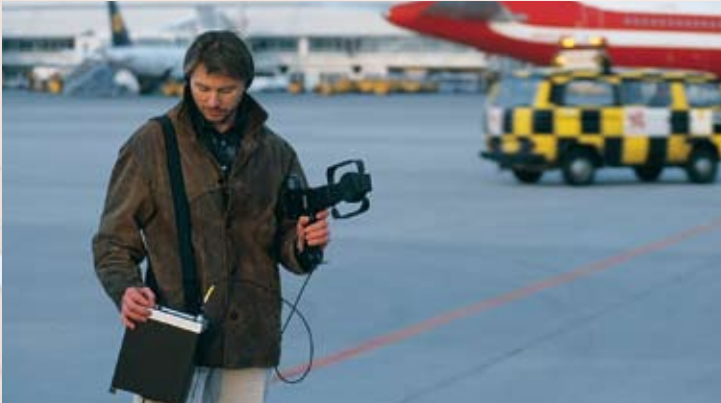
Searching for interference sources in areas with sensitive equipment
