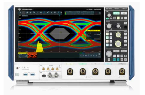
Eye diagrams give a quick overview of data signal jitter and noise while also revealing the robustness of data transmissions. Numerous fast bus interface standards, such as USB and PCI Express (PCIe), now define eye masks for signal integrity testing, clearly illustrating their importance.
