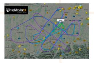
The first MICONAV test flight was routed over four LDACS ground stations that were specially set up for this project in southern Bavaria. Two of the stations had transmitters for collecting navigation data. The other two had transceivers for digital aeronautical radio data. The flight paths were planned to allow testing of the handover process (top left) as well as various triangulation scenarios using two to four ground stations (bottom left).
