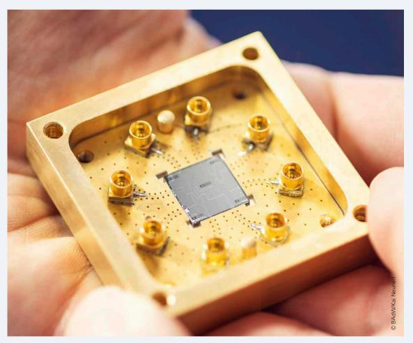
Fig. 1: Manufactured at the Walther-Meißner-Institute: the chip in the RF housing has several superconducting circuits.
