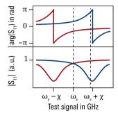
Fig. 2: The two systems mutually influence each other through the interaction between the qubit and resonator (left). Depending on the qubit state (blue and red curves), the resonance frequency  $\omega_r$  shifted by a certain modulus  $\chi$ . Using a test signal, the transmission and reflection properties of the resonator can be determined – and thus the state of the qubit. The argument and modulus of the S-parameter S<sub>11</sub> are plotted on the right.
