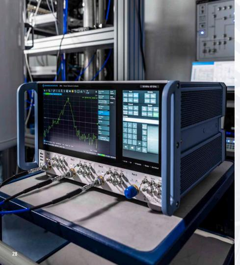
Fig. 3: Measurement setup at the Walther-Meißner-Institute with a cryostat (right) and an R&S<sup>®</sup>ZNA vector network analyzer (left) for analyzing the resonances of superconducting circuits.
