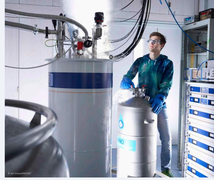
Fig. 2: Cryostats like this one hold superconducting circuits operating at temperatures close to absolute zero.
