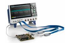
The new R&S®MXO 4 oscilloscope with mixed signal option (MSO) and DUT (page 38).
