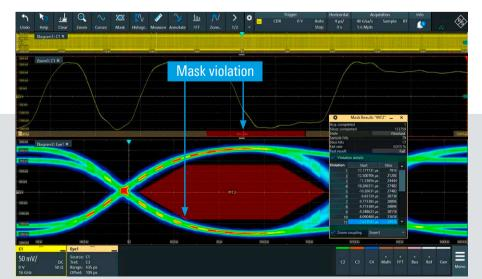
Fig. 1: The eye stripe function makes debugging much easier. Mask violations are marked in red in the eye diagram and in the time signal of the waveform (blue arrows). All violations are listed in the results table and the currently displayed signal section is marked in blue.
