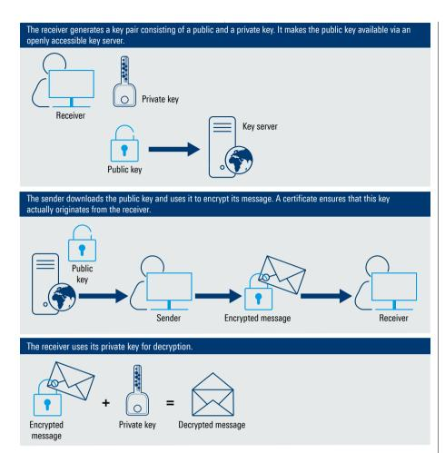
Fig. 1: Basic principle of asymmetric cryptography.
