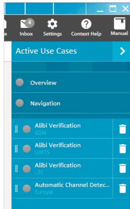
In the alibi verification area, the measurement parameters can be configured for the appropriate frequency range (Fig. 9): this is where the parameters from the templates are displayed. They can be modified if necessary.
