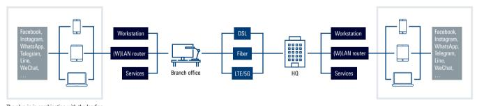
The plug-in in combination with the leading DPI engine R&S®PACE 2 detects NATing and devices behind the corresponding routing device, and the applications used.
