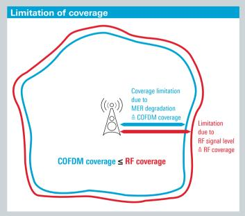
What is the required minimum transmitter MER? Transmitter coverage is defined by the transmission loss down to the noise level (= RF coverage). Moreover, MER degradation affects digital COFDM signals. Consequently, COFDM coverage ends where minimum receiver MER requirements are just being met. Since RF coverage is the dominant physical characteristic, increasing the transmitter MER allows the COFDM coverage to be extended only up to the RF coverage limit.
