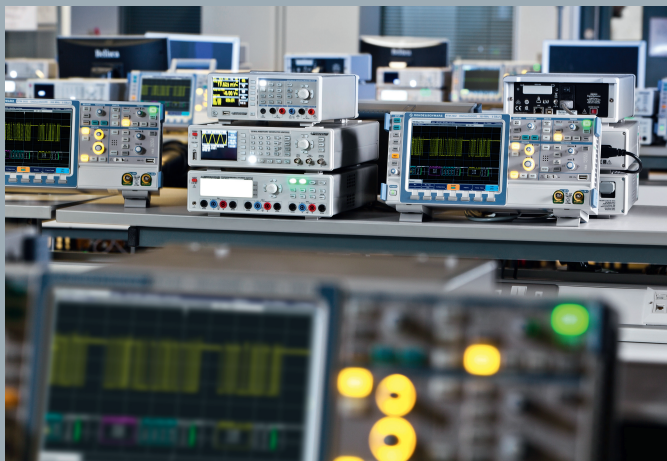
A typical workstation consisting of an Oscilloscope, Function Generator, Power Supply and Multimeter.
