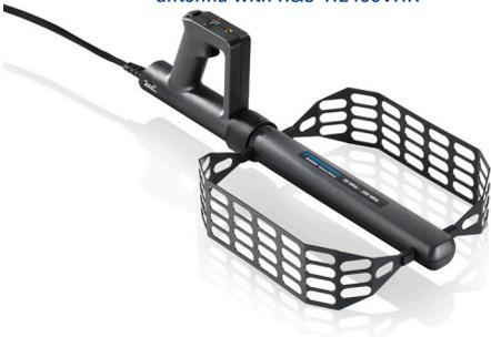
The R&S®HE400 antenna handle has an operational frequency range from 8 kHz to 8 GHz and supports all antenna modules up to this frequency. It is compatible with the R&S®PR200 portable monitoring receiver, the R&S®Spectrum Rider FPH handheld spectrum analyzer (models .02/.06), the R&S®FSH4 and R&S®FSH8 handheld spectrum analyzers and the R&S®CableRider ZPH cable and antenna analyzer (model .12).<sup>1)</sup>
