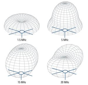
Typical gain on a 5 m mast above perfectly conducting ground
