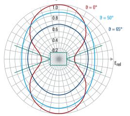
Typical vertical radiation pattern (12 m above an ideal conductive plane)
