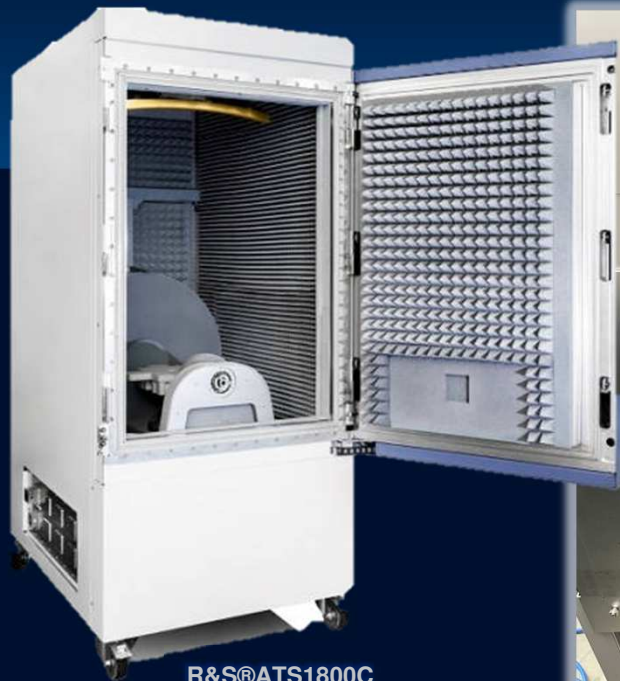
R&S@ATS1800C Compact 3GPP-compliant OTA chamber for 5G NR mmWave signals
