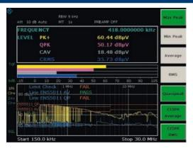
Menu for selecting weighting detectors. Values produced by a maximum of four different detectors are simultaneously displayed, both numerically and as an analog bargraph
