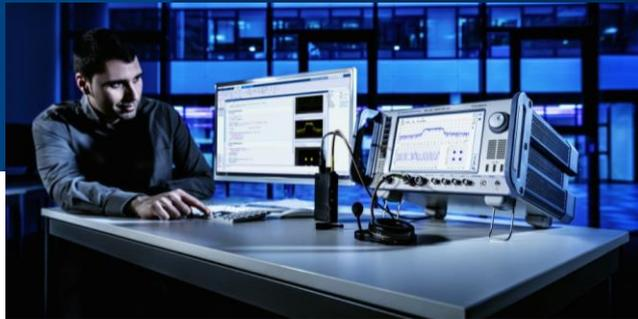
The QuickTune software solution for R&S®CMArun supports fully automatic testing and tuning of most commonly used LMR radios. LMR radios can be reliably tested, aligned and serviced by connecting the R&S®CMA180 to the radio and initiating the R&S®CMArun and QuickTune sequences. No further user interaction is required.
