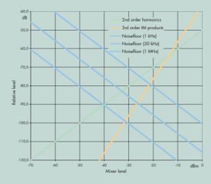
Dynamic range, noise, and 1 dB compression point of Signal Analyzer FSIG3
