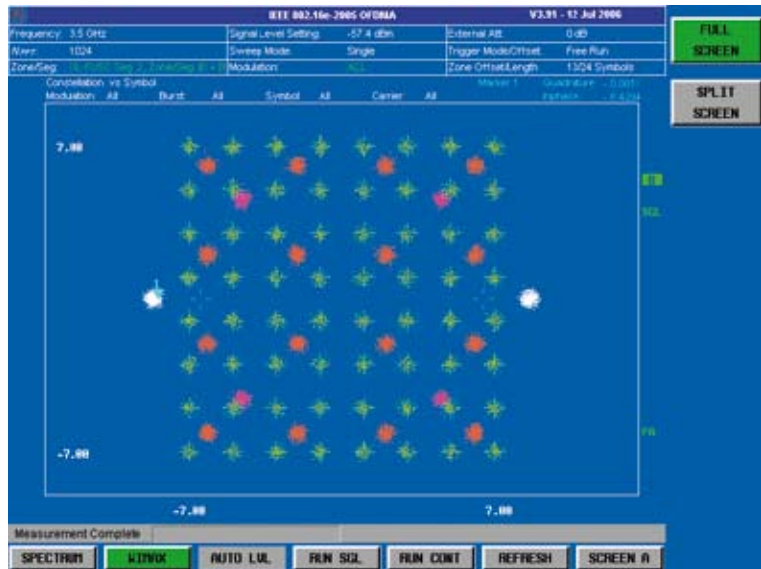
Constellation diagram with low signal-to-noise ratio.
