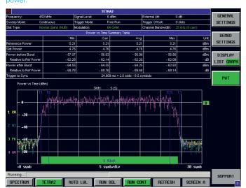
Adjacent channel power (ACP) measurement: The bandwidth of the TX channel depends on the number of carriers; the power in the adjacent channels is determined by means of a TETRA filter.
