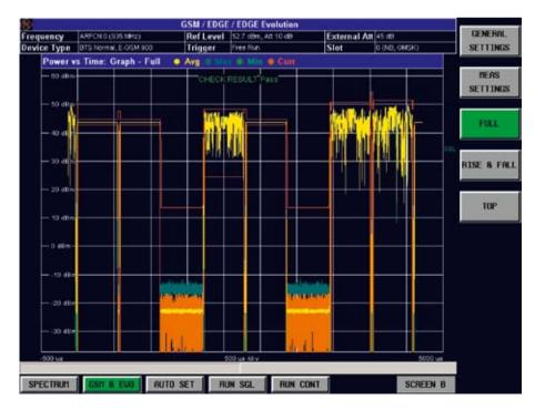
The power versus time measurement allows both single- and multi-slot analysis using fully standard-conforming limit lines. The limit lines are automatically configured based on the measured slot powers, burst types and device parameters, e.g. device type and power class.
