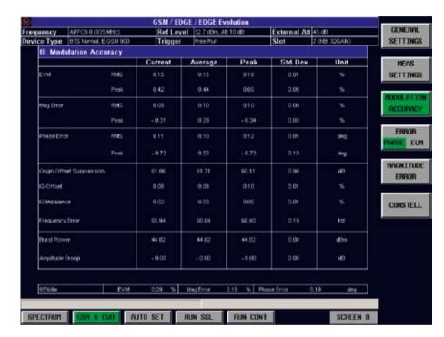
The Modulation Accuracy table provides an overview of the most important modulation parameters at a glance. Statistics are calculated based on a configurable number of bursts. All standard-required parameters plus additional values such as I/Q imbalance are measured.
