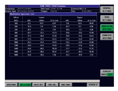
The Modulation Spectrum measurement in List mode automatically compares the standard-specified frequencies to the appropriate limits.
