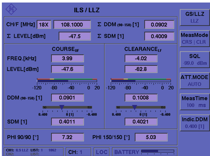
Simultaneous analysis of course and clearance signals.
