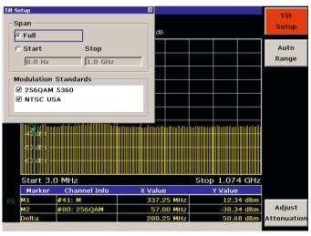
Frequency spectrum of a J.83/B signal with interferer
