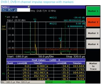
Channel impulse response with SFN frequency offset measurement (red lines)
