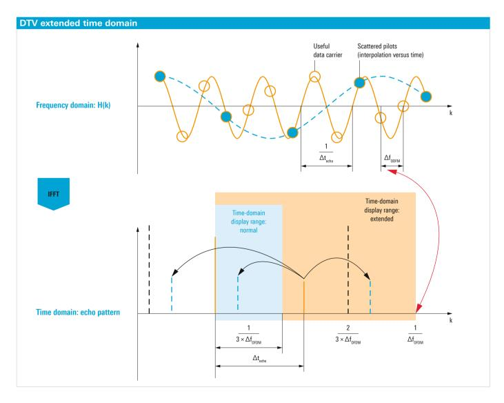
A special feature of the R&S®ETL is the positioning of the FFT window. To help ensure stable synchronization to the transmitter signal, especially for field measurements, the R&S®ETL tries to place all impulses above an echo detection threshold so that they are equidistant within the guard interval. For some applications, the echo detection threshold is dependent on the system optimization method selected by the user.
