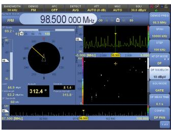
DF result shown using a DF compass rose and azimuth diagram.
