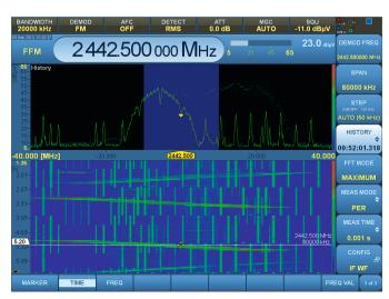
Strong activity in the 2.4 GHz ISM band caused by WLAN and Bluetooth® signals (superimposed in frequency and time; can be unambiguously identified using the realtime spectrum).
