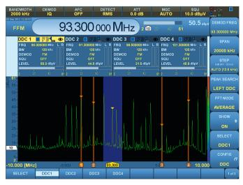
4+1 demodulation channels with different parameters within the realtime bandwidth.
