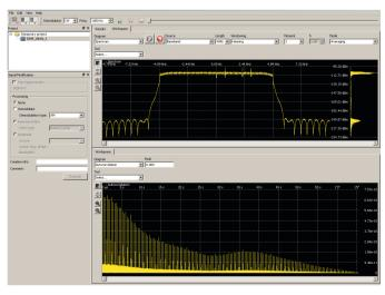
Offline measurement of a Digital Radio Mondiale (DRM) signal in line with ITU-R SM.1600.
