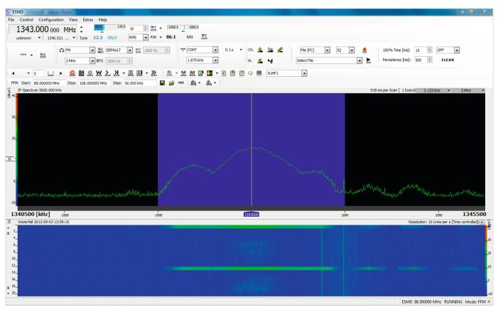
Realtime spectrum and waterfall display of a radar signal from Munich airport.
