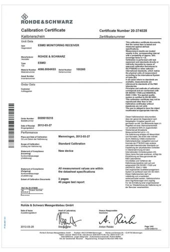
Documentation of calibration values; example of an R&S°ESMD-DCV calibration certificate (cover sheet).
