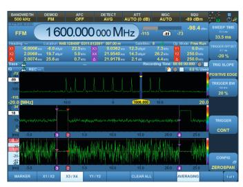
Measurement of a frequency hopping signal. The markers can also be used to measure intervals (center) and the instantaneous frequency (bottom).
