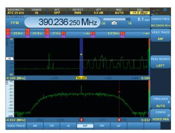
Transmission rate estimate of a TETRA signal using a squared video spectrum (signal peaks approx. 18 kHz from center frequency; transmission rate approx. 18 kBd).
