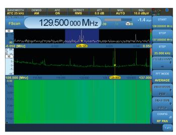
For audio demodulation, the ATC radio band is examined in 25 kHz steps to detect signals that exceed the squelch level.
