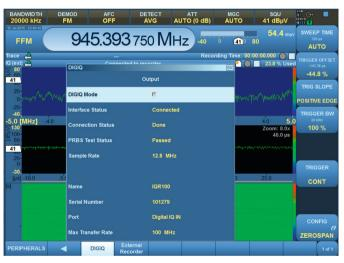
Status report for an R&S°IQR100 connected to the R&S°Digital I/Q Interface.
