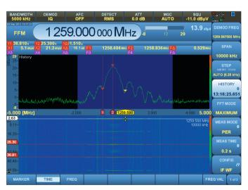
1259 MHz radar signal from Munich airport; determination of simple parameters using spectrum and waterfall.
