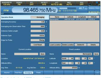
Detailed display of GPS data and GPS operating mode.
