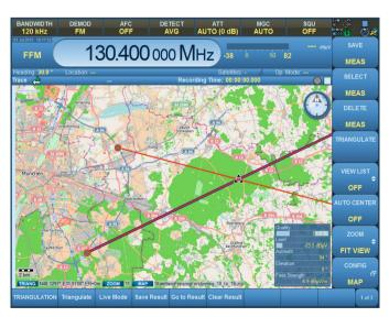
The positions recorded during a drive test (including the bearing, if applicable) are shown on a map.
