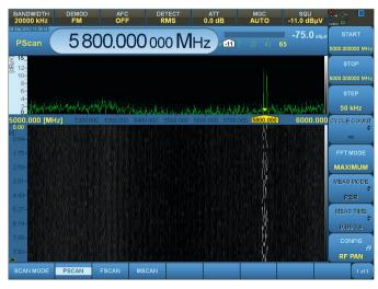
Detection of a hopper signal in the 5.8 GHz ISM band using the fast spectral scan over the 1 GHz bandwidth.
