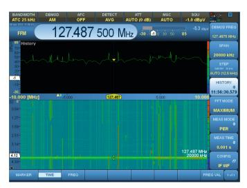
Strong wideband interference is superimposed on the entire aeronautical radio band.
