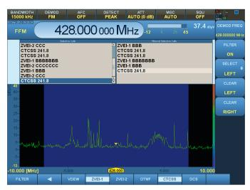
Display of detected selective call standards in an overview list (left column); filtering by relevance possible (right column).
