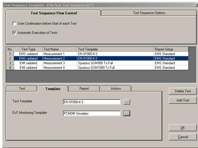
Intuitive operation owing to virtual instrument concept: example of an EMI measurement within a test sequence.
