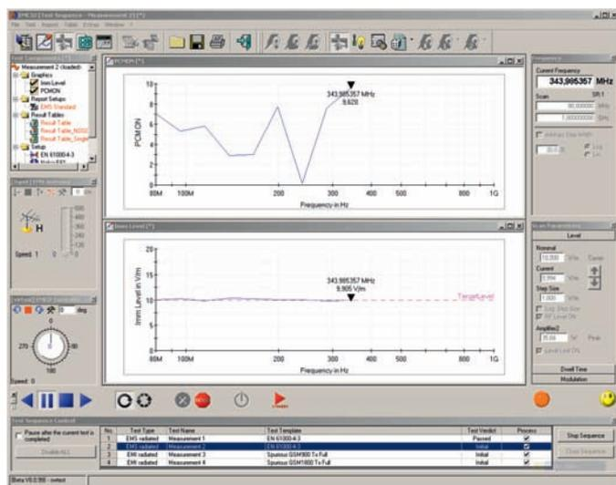
Interactive test sequence flow control of automatic test sequences.
