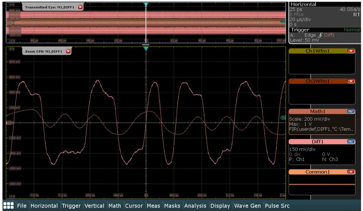
During root cause analysis, the R&S®RTP oscilloscope provides support with analysis tools such as eye diagrams with mask tests or separation of jitter and noise components. Time domain reflectometry is also available for verifying the transmission characteristics of passive signal path components such as connectors, cables and signal lines on the printed board.
