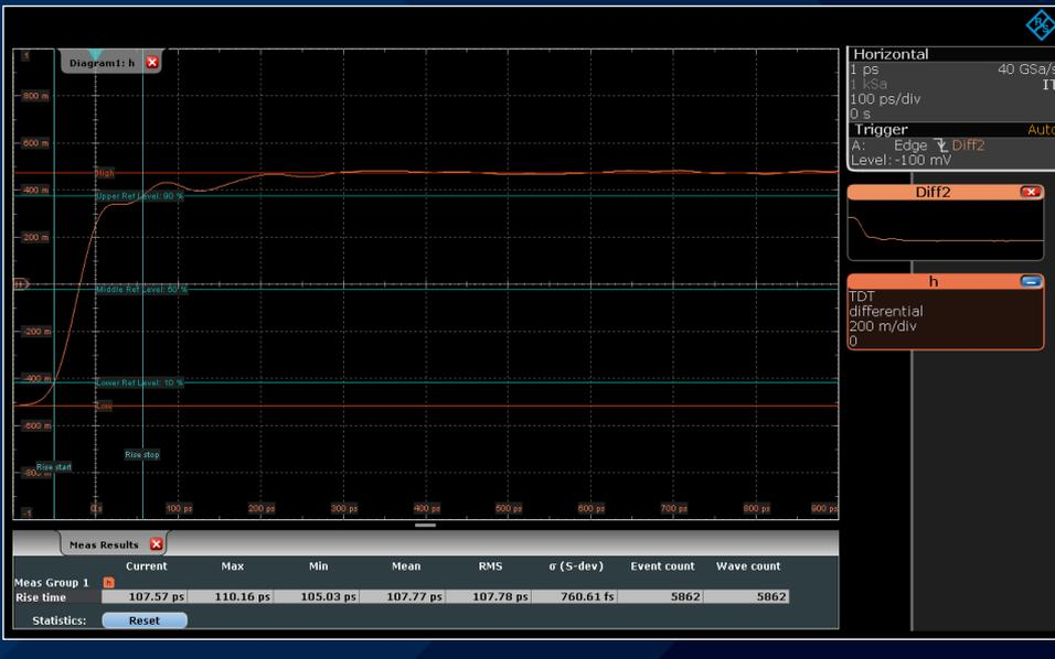
Time domain transmissometry (TDT) is another useful measurement capability. Here, a fast pulse is also fed into the signal path. The output is connected to the oscilloscope channel to allow determination of the transmission losses. The TDT result shows the pulse shape that arises due to transmission losses. The rise time measured in the example in Fig. 12 suggests a bandwidth of about 3.2 GHz ( $BW = 0.35/t_{rise}$ ).
