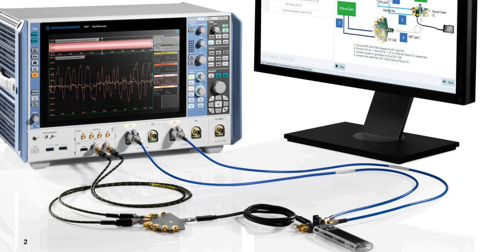
Fig. 2: Acquisition of the “short channel” trace for a USB 3.2 Gen 1 device on channels 1 and 3 with real-time calculation as a differential signal (Diff 1). Calculation of the “long channel” signal through embedding of the S-parameters through the USB-IF (Math 1).
