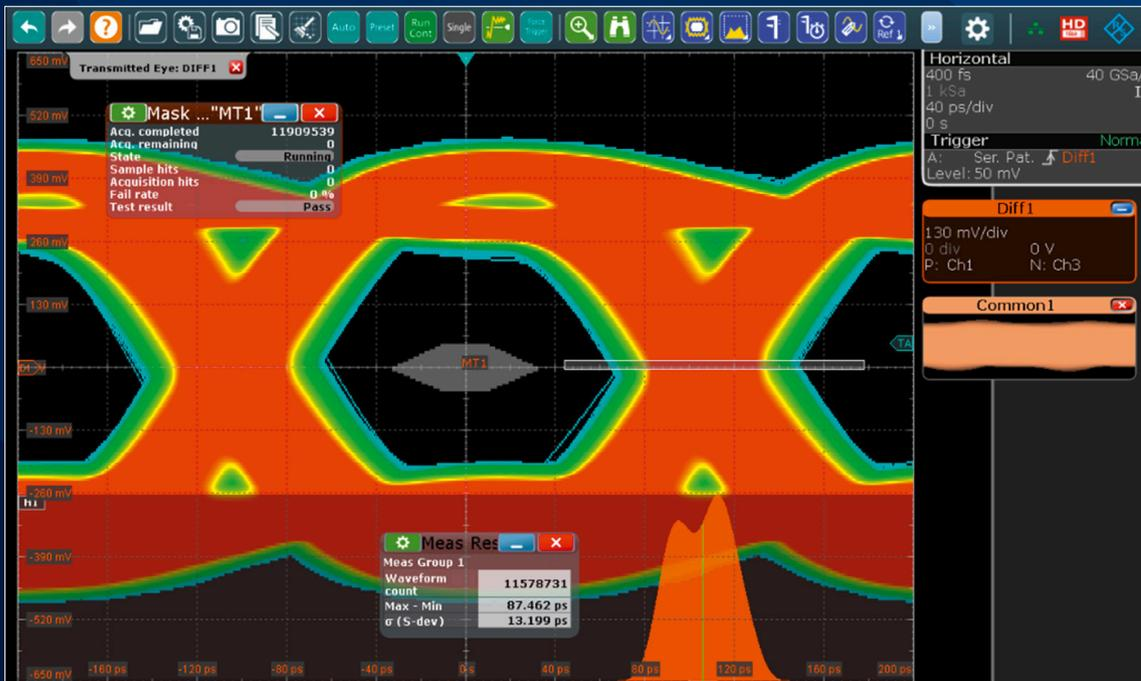
Fig. 6: Real-time eye pattern for the faulty USB device using hardware based CDR, mask testing and histogram with the R&S®RTP164 oscilloscope.
