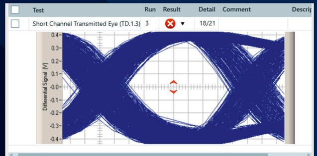
Fig. 4: The eye pattern is produced by superimposing bit sequences.
