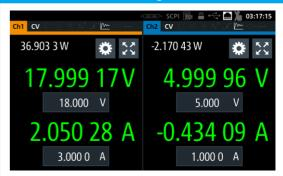
A resolution of up to 61/2 digits is perfect for characterizing DUTs that have low power consumption in standby mode and high current in full load operation. The R&S®NGL200 power supplies automatically switch from source to sink mode. Operating as a load is indicated by a negative current reading.
