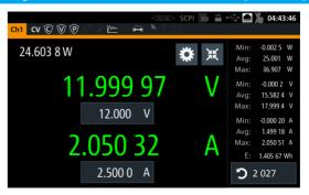
The large capacitive touchscreen is the central operating element. With its very high resolution of 800 x 480 pixel, the display makes it easy to read the voltage and current fields even at great distances. Additionally, information such as power values or statistics can be displayed. Icons clearly show the status of the set protection or special functions.
