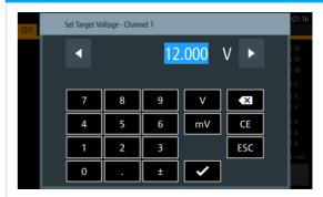
The large capacitive touchscreen is the central operating element. Lightly tapping a numerical value brings up a virtual keyboard to enter the desired value. Alternatively, voltage, current and limits for the various protection functions can be set using the rotary knob.
