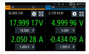
A resolution of up to 6 ½ digits is perfect for characterizing DUTs that have low power consumption in standby mode and high current in full load operation. The R&S\*NGL200 power supplies automatically switch from source to sink mode. Operating as a load is indicated by a negative current reading.
