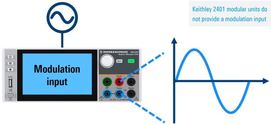
The R&S®NGU401 source measure unit provides a modulation input to connect an arbitrary generator, for instance. The output follows the modulation input signal, enabling the instrument to act as an AC source and be used to simulate glitches and unstable conditions.
