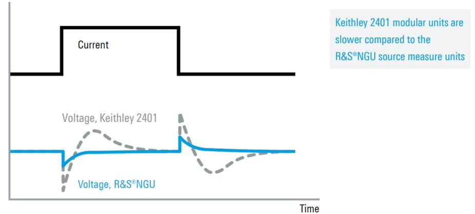
Under challenging load conditions, most power supplies respond with slow recovery times and overshoot. Specially developed circuits in the R&S®NGU source measure units achieve a load recovery time of  $< 30 \mu\text{s}$  with minimal overshoot, making them perfect for supplying sensitive components with power.
