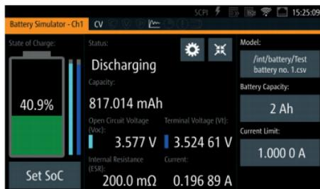
Capacity, open circuit voltage (Voc) and equivalent series resistance (ESR) are important battery characteristics that are based on the battery's state of charge (SoC). The optional R&S®NGM-K106 battery simulator allows users to simulate battery behavior under different charging conditions, such as when powering a DUT.
