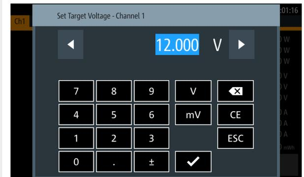
The large capacitive touchscreen is the central operating element on the R&S®NGM200. Lightly tapping a numerical value will display a virtual keyboard to enter the desired value. Alternatively, the rotary knob can be used to set voltage and current values as well as limits for the various protection functions.
