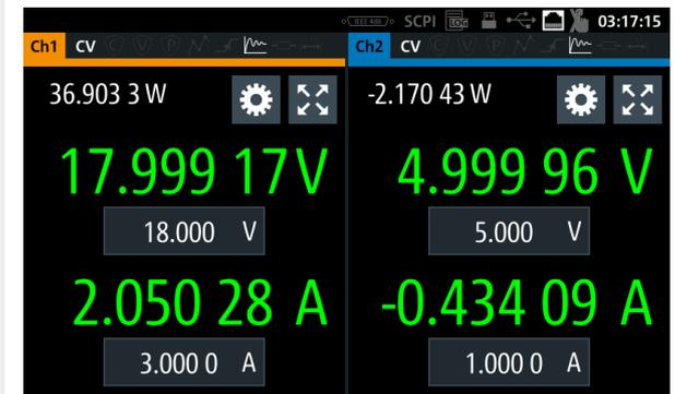
A resolution of up to 6½ digits is perfect for characterizing DUTs that have low power consumption in standby mode and high current in full load operation. The R&S®NGM200 power supplies automatically switch between source and sink mode. A negative current reading indicates that the instrument operates as a load.
