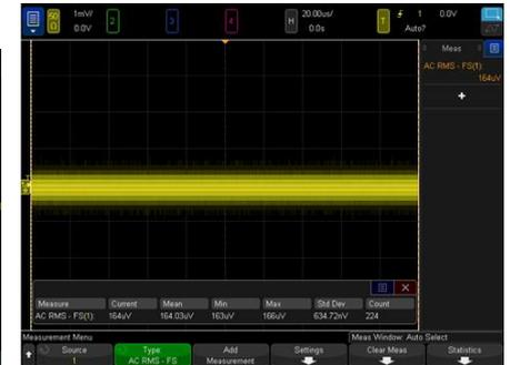
The 4000 X-Series has 5 times the noise of the R&S®RTA4000. Higher noise lowers the accuracy of measurements and makes it more difficult to see small details.
