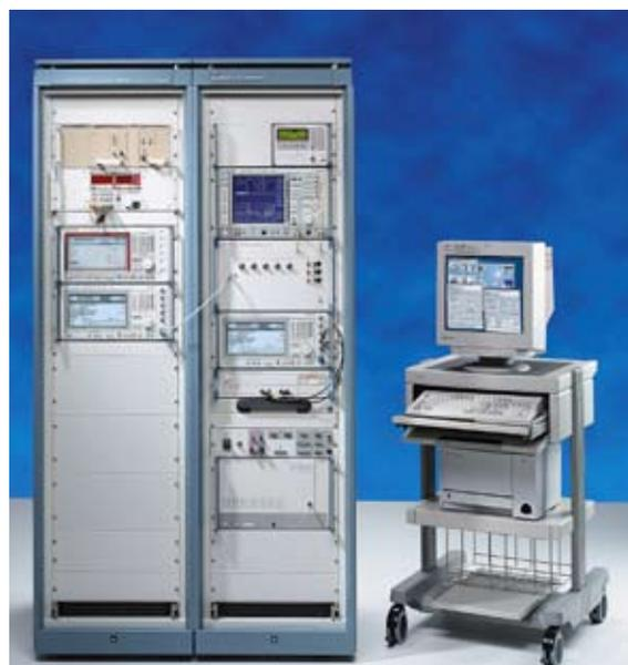
*2G/3G conformance testing with the R&S®TS895xGW family*
