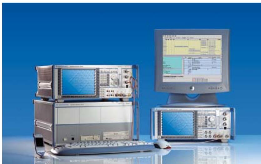
*Test solution for 2G/3G intersystem handover*
