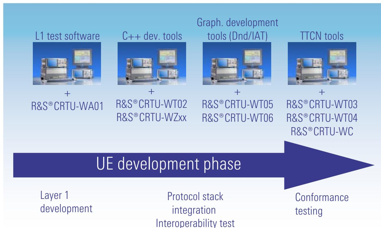
*The R&S®CRTU-W can be configured to meet any development requirements*
