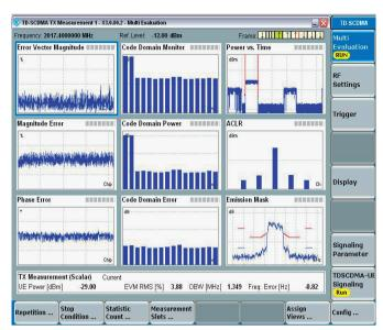
Based on data sets of identical signal samples, the R&S®Multi-Evaluation measurement allows the simultaneous evaluation of a variety of signal parameters, such as transmitter output power and spectrum measurements, i.e. spectrum emission mask (SEM) and occupied bandwidth (OBW), as well as modulation accuracy measurements, i.e. error vector magnitude (EVM) and more, in nonsignaling and signaling mode.
