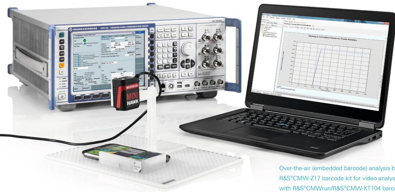
Over-the-air (embedded barcode) analysis based on the R&S®CMW-Z17 barcode kit for video analysis in combination with R&S®CMWrun/R&S®CMW-KT104 barcode video analysis.
