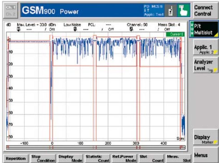
*The R&S®CMU200 can also measure spectra, power, and modulations. Here is an example of a power measurement during a file transfer with four slots in the uplink and triggering in response to combined GMSK/8PSK modulation.*
