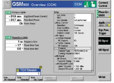
The signaling mode overview menu informs the user quickly and comprehensively about the BTS's TCH RF performance; timeslotselective measurements are possible.
