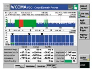
Code domain power (CDP) measurement on a HSDPA signal containing 5 × HS-DSCH and 4 × HS-SCCH channels. The R&S<sup>®</sup> CMU 300 automatically demodulates QPSK or 16QAM codes and includes them in the code domain analysis.
