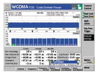
Peak Code Domain Errror (PCDE) measurement on a HSDPA test model.
