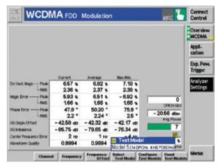
Composite Error Vector Magnitude (EVM) measurement on a HSDPA test model.
