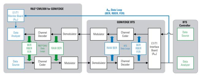
Setup for BER Testing.
