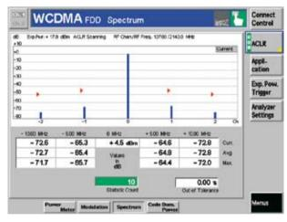
Adjacent Channel Leakage Ratio (ACLR) measurement.
