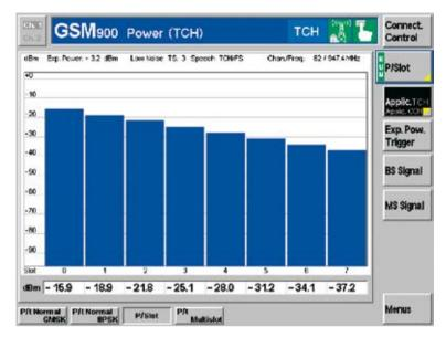
Power versus slot measurement.
