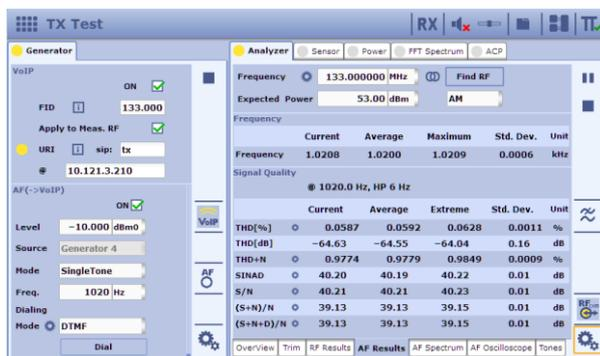
R&S CMA180: The VoIP audio generator provides the IP connection and the audio input to the radio. The radio will modulate the digital audio signal and transmit it to the R&S CMA180 over the air interface. The R&S CMA180 then measures the RF parameters and the signal quality.
