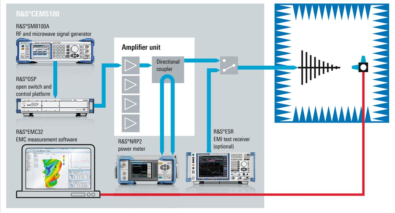
The R&S®CEMS100 includes all the components required in an advanced EMS test system:
