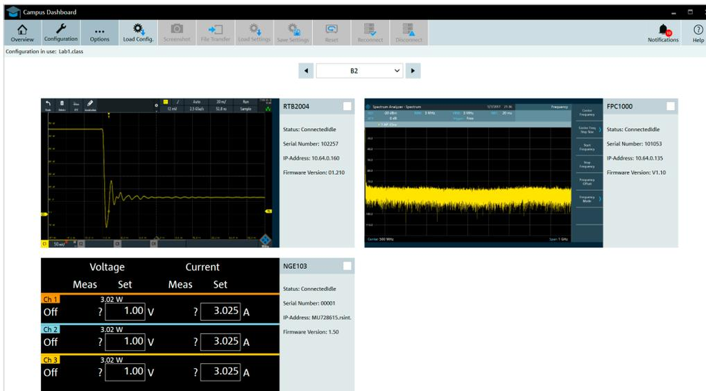
View all instruments on a bench on your computer screen using the R&S®CDS campus dashboard software; the software also supports remote control of each instrument
