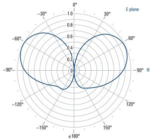
Typical vertical radiation pattern at 1.1 GHz
