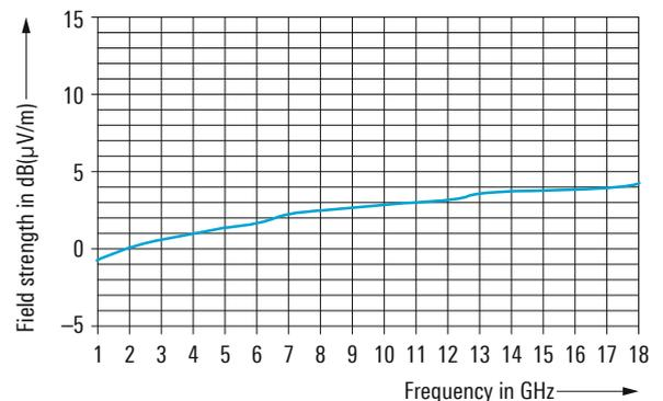
With R&S®HL024S9 (for a receiver with  $F = 15$  dB,  $\Delta f = 1$  MHz).
