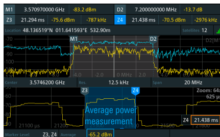
Fig. 4: Average power measurement
