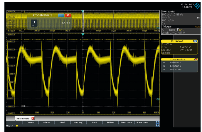
Comprehensive screen on the oscilloscope zooming into a longer period of recording.
